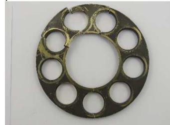
Retaining plate contact slipper pad
